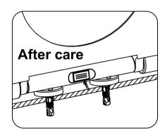
For cleaning, press the middle button just with one finger and take off the seat. Clean the seat and other desired area, and then reattach the seat onto the hinge pins.
